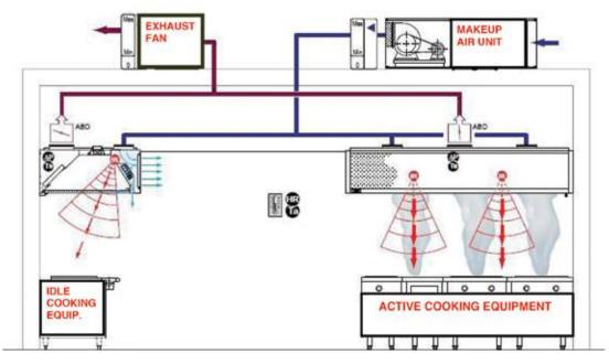
*Figure 9. Schematic DCKV system showing infrared sensor activation control with active and idle cooking equipment. Halton Group.*
