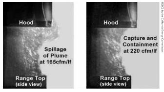
*Figure 2. Schlieren images of hoods at different exhaust rates per linear foot (lf).*
