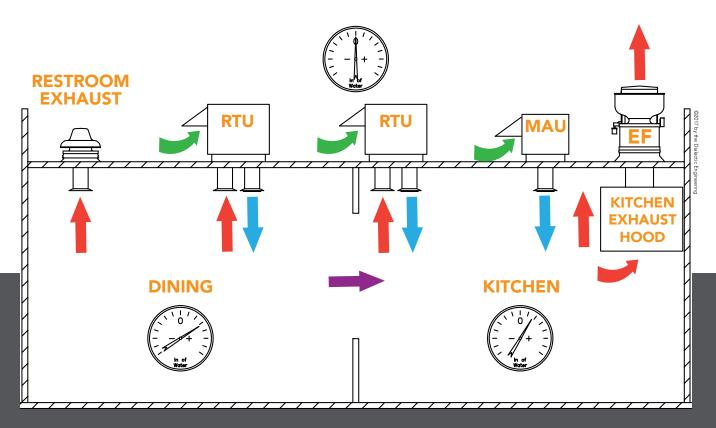
Figure 1: Schematic of a common commercial food service ventilation configuration
