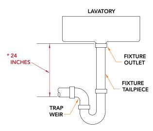
\*MAXIMUM DISTANCE FROM FIXTURE OUTLET TO TRAP WEIR
